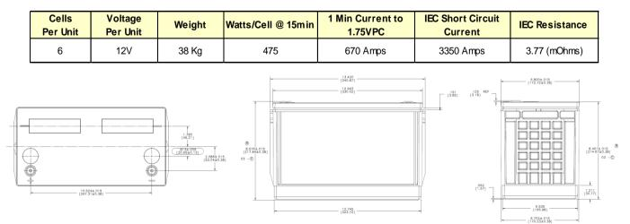
\*All dimensions in inches and (millimeters). All dimensions are for reference only. Contact a C&D Representative for complete dimensional information.
